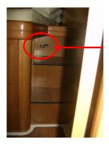
The 2 fuel tanks on Sea Vous Plait hold a total of 180 gallons of diesel. To change from one tank to the other simply locate the change over lever in the starboard aft cabin (it is on the top step to the right of the bunk) and either push it in or pull it out depending on its original position.
