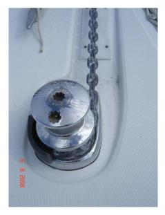
To drop the anchor, insert your windlass handle into the central opening on top of the windlass.
