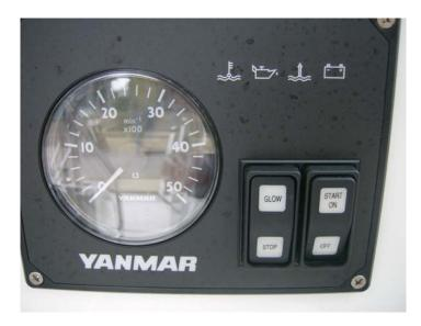
Should you hear an engine alarm during operation, check which light is on and immediately shut down the engine-CALL HORIZON
