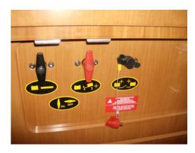
In the port aft cabin you will find the port engine battery breakers and the parallel starter.
