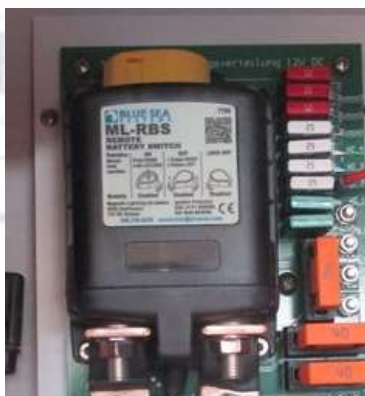
House battery isolator behind port salon seating
