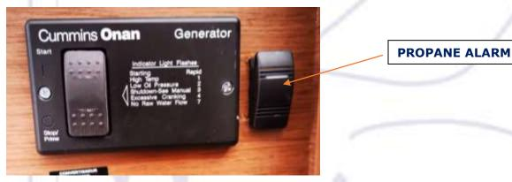
The 12v solenoid system is USCG approved device. You do not need to shut any manual valves unless you wish.
