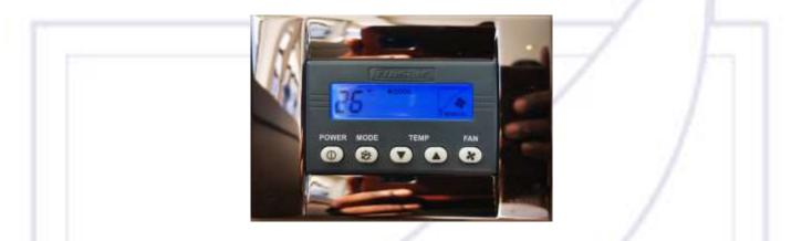
The air conditioning units should be turned on **after** the generator has been running for 5 minutes (or once the boat is plugged into shore power) and the breakers should be shut **off** before stopping the generator or unplugging from shore power.
