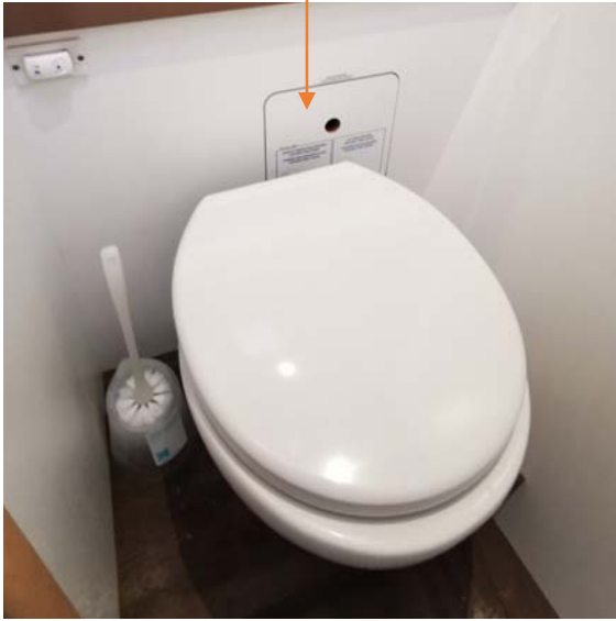
Port Holding tank seacock in main shower
