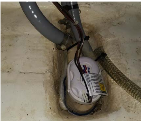
Fully automatic bilge pump below saloon floorboard
