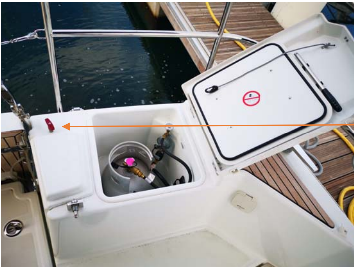
Pull cord to activate generator fire extinguisher
