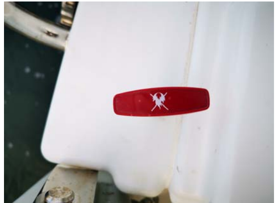
Pull cord to activate generator fire extinguisher
