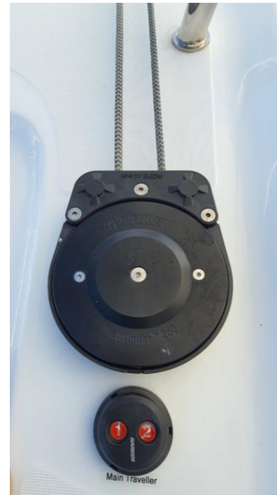
Two-way winch for travellers
