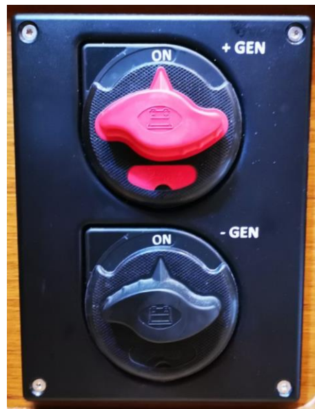
Generator Battery Switch
