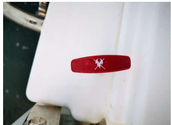
Pull cord to activate generator fire extinguisher
