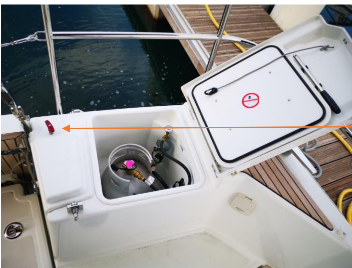
Pull cord to activate generator fire extinguisher
