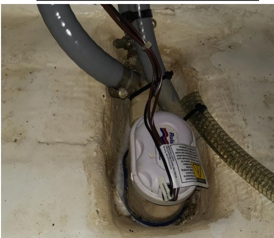
Fully automatic bilge pump below saloon floorboard
