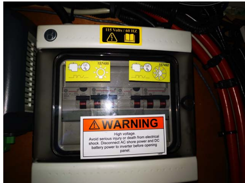
Generator/Shore power 110V breakers in Stbd lazarette
