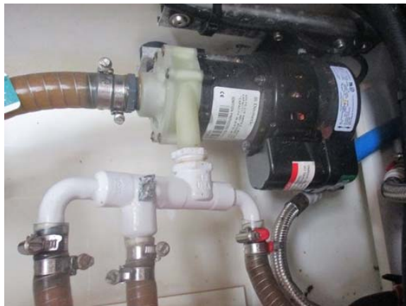
Ac pump under saloon floorboard (saloon and aft)
