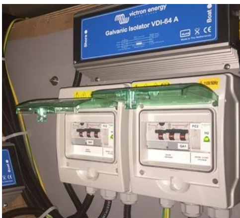
110V Breakers under stbd aft cabin bunk (remove mattress for access)
